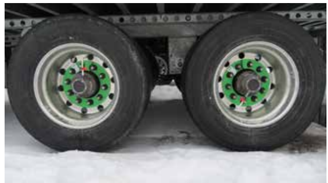
LWS Sensor Rings installed on dual axial trailer
