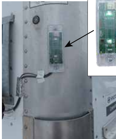
LWS Alarm Beacon mounted on front of trailer
